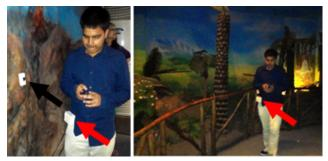
Figure 1: User navigating with the aid of the system. User module (red arrow) and wall module (black-arrow). Left image is the start position of the exhibition.
